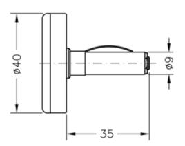
Bi-metal thermometer with rear stem, galvanized casing and embossed glass; particularly suitable for under-floor heating systems.
