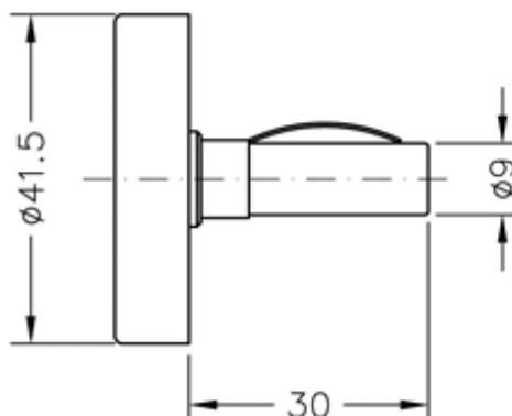
Bi-metal thermometer with rear stem, galvanized casing and nickel-plated glass retainer; particularly suitable for under-floor heating systems.
