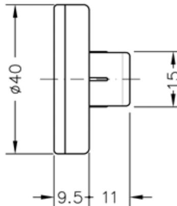
Bi-metal thermometer with rear stem and single body in plastic material; particularly suitable for under-floor heating systems.
