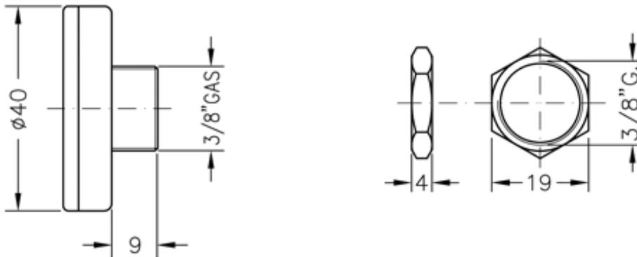
Bimetal thermometer with threaded rear stem and fixing nut, plastic casing and embossed glass; particularly suitable for refrigerating cells, display cabinets and cold counters.
