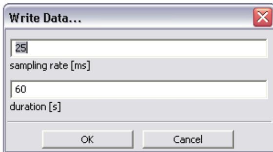
In the dialog the interval between the measurements (sampling rate in milliseconds) and the overall duration (duration in seconds) can be specified. As soon as "OK" is pressed, the recording is started.
