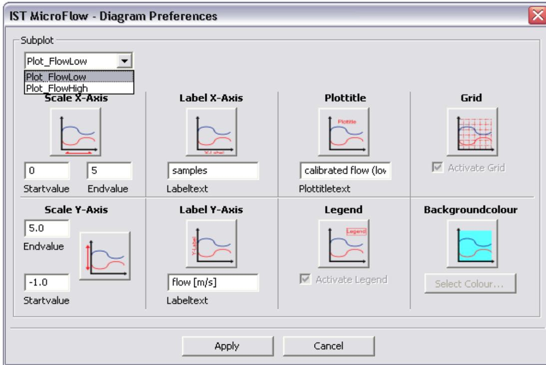
The two output modes Flow\_Low und Flow\_High can be chosen in the dropdown menu. With Flow\_Low the flow value is calculated from the voltage at the flow sensor. With Flow\_High the flow value is calculated from the voltage URight. Flow\_Low can be calibrated over the parameters in 4.4 and Flow\_High with the parameters in 4.3.
