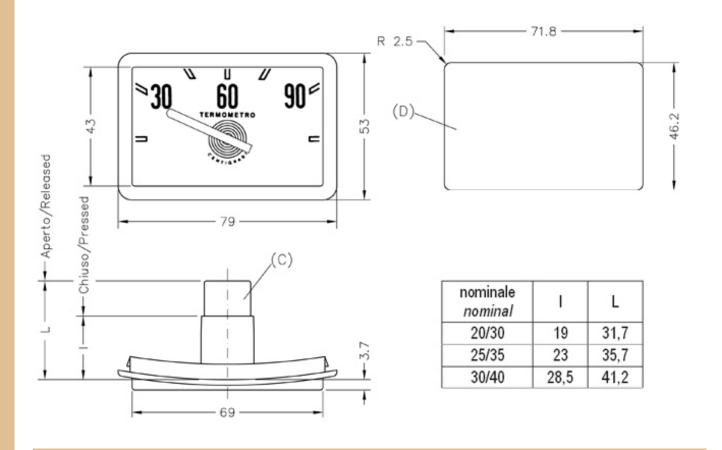
Bi-metal contact thermometer for water heater, with embedded fixture on rectangular hole.
